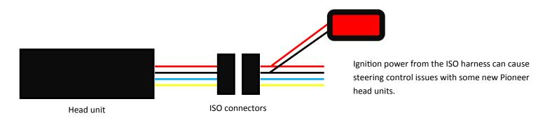
Some new Pioneer head units do not respond correctly to the steering controls. This is due to a voltage supply issues from the car to the interface.
